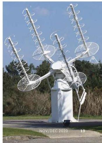
Circularly polarized antennas transmit (and receive) signals with polarities that rotate as they travel. This is an array of four circularly polarized antennas used for space communication.
